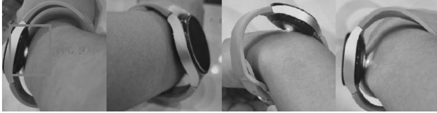
〈Figure 3〉 Experimental setup with a PPG sensor in wearable smartwatch devices to wrist positions towards various postures
