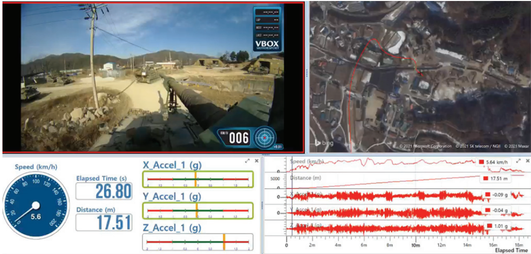
〈Figure 3a〉 An example of condition monitoring system during K9A1 driving 26)
